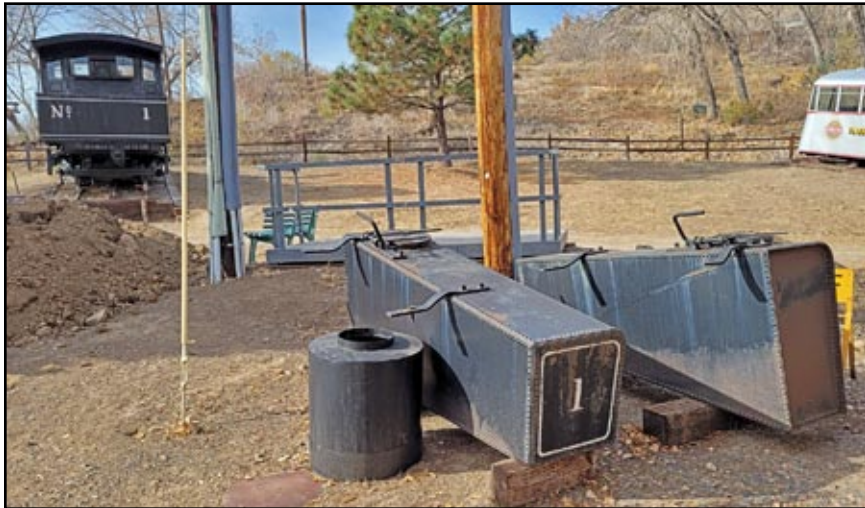
The saddle tanks from the Manitou & Pikes Peak cog steam engine No. 1 at the Colorado RR Museum have been removed for engine and boiler maintenance. – Photo © 2022 Dave Schaaf.
