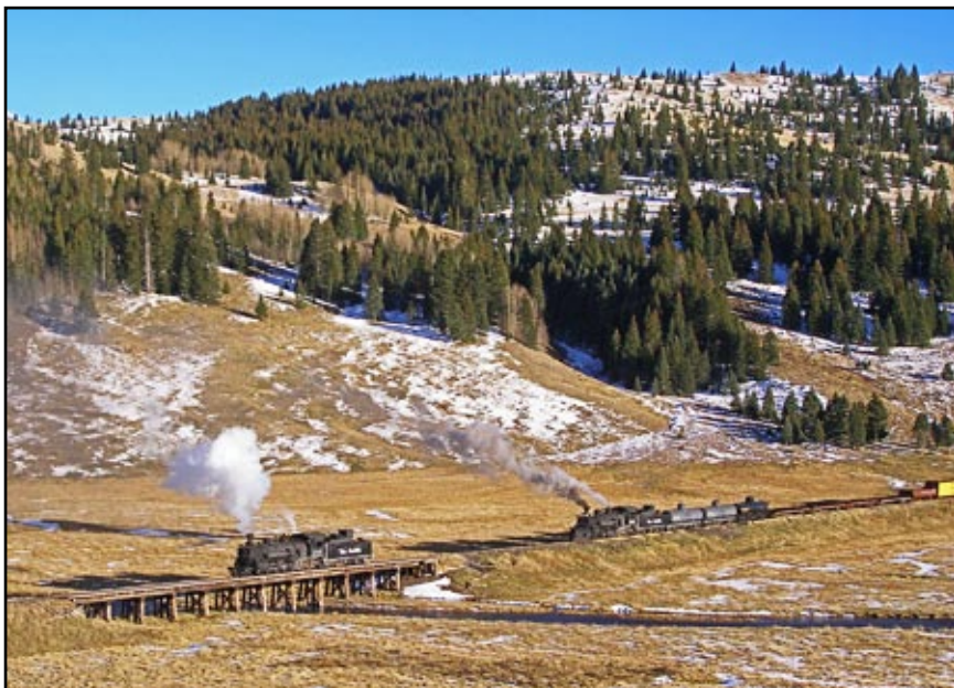
Locomotive #484 decoupled from its train before crossing the Los Pinos trestle and running light to the water tank. – Photo © 2006 Keith Jensen.
