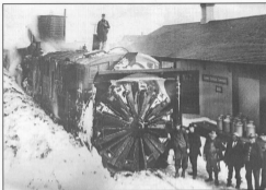
C&S rotary No. 99201 was used to clear the mainline between Cheyenne, Wyoming, Denver and Falcon, Colorado. It paused at Elizabeth, Colorado to take on water and pose with its crew.
